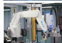
Articulated robots applied for function tests for SCARA robots to shorten testing time
